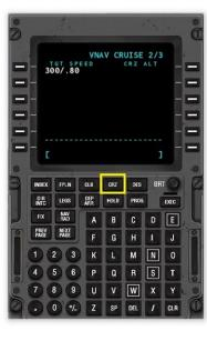
Input the cruise altitude into the scratch pad.
