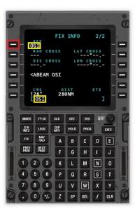
Input the desired radial (038) into the scratch pad.
