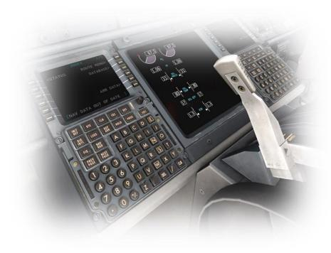
A Flight Management System (FMS) is a centralized computer system used in airliners, and other high-performance aircraft, to manage many of the aircraft systems, including (but not limited to) the flight plan.
