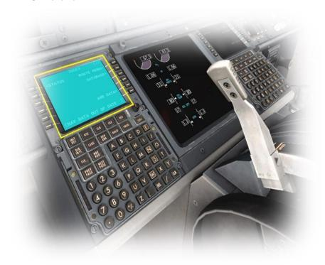
To invoke the pop-up CDU panel, position and click the mouse-pointer anywhere inside the **DISPLAY** area of the CDU panel in the 3D cockpit.
