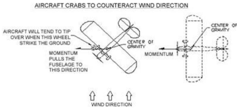
Figure15b : Tricycle Type in a Cross Wind Landing
