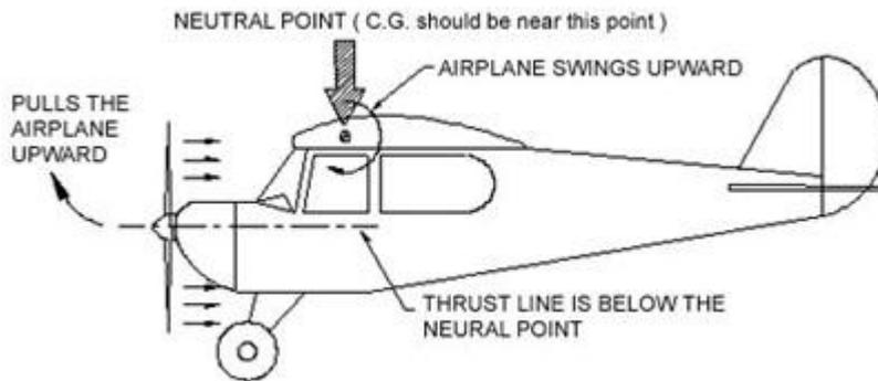
Figure13b : Side view of model aircraft engine with 3 degrees down thrust
