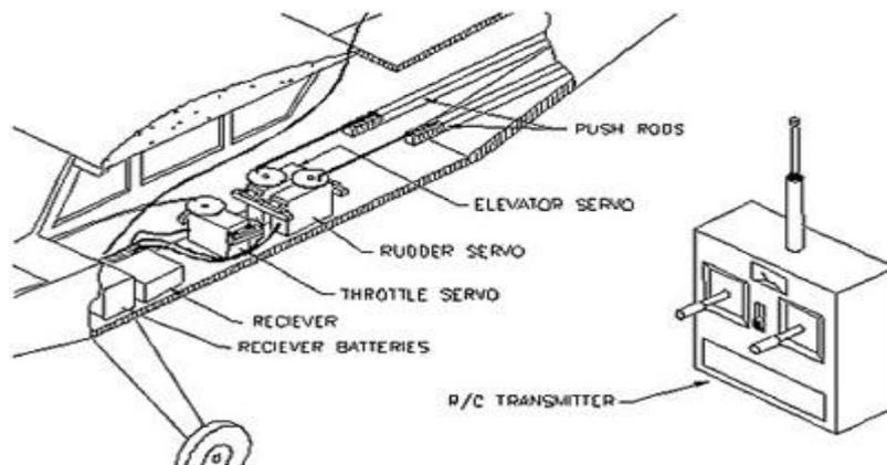
**FIGURE 3b : Typical four-channel radio control layout and components**
