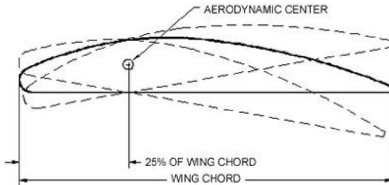
**Figure 16b : Neutral Point of Wing and Horizontal Stabilizer**
