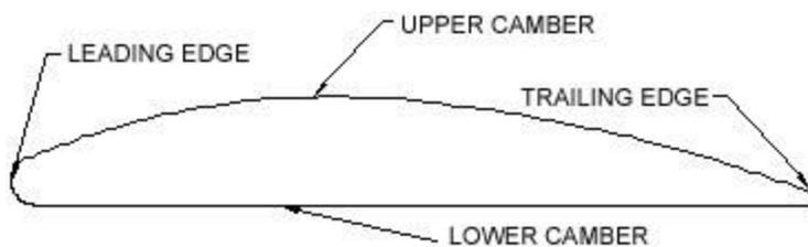
**Figure 4b : Airfoil of a typical rc airplane**
