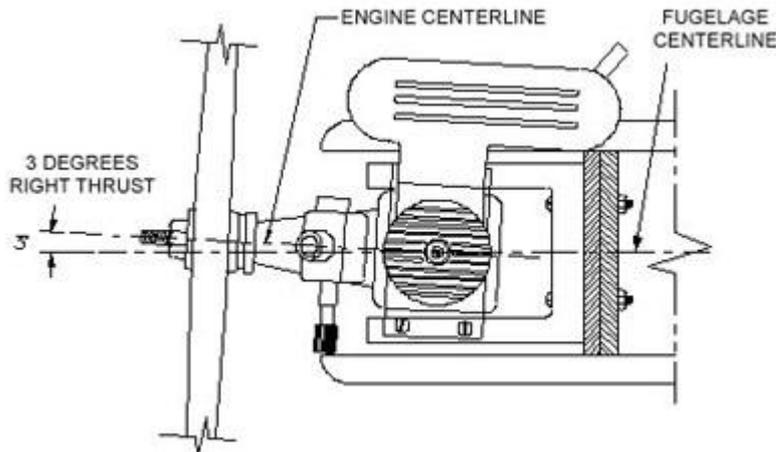
Figure 12b : Illustration of engine vs. propeller torque
