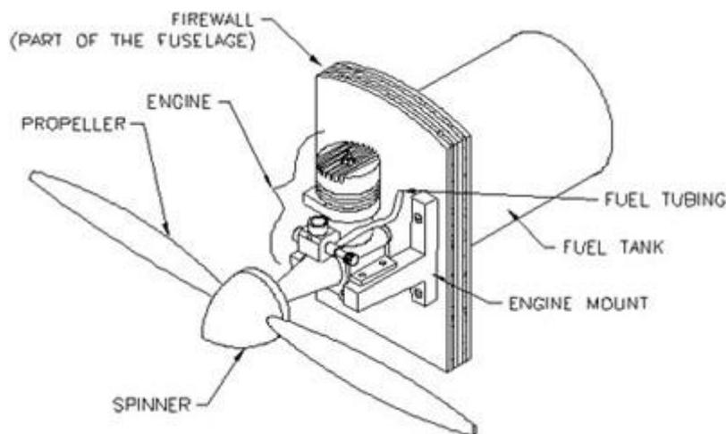
Usually the model aircraft use three different types of internal combustion engines with regards to the fuel they use.
