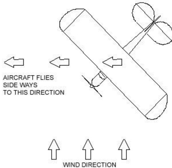
Figure14b : Aircraft deviates from straight path in a crosswind
